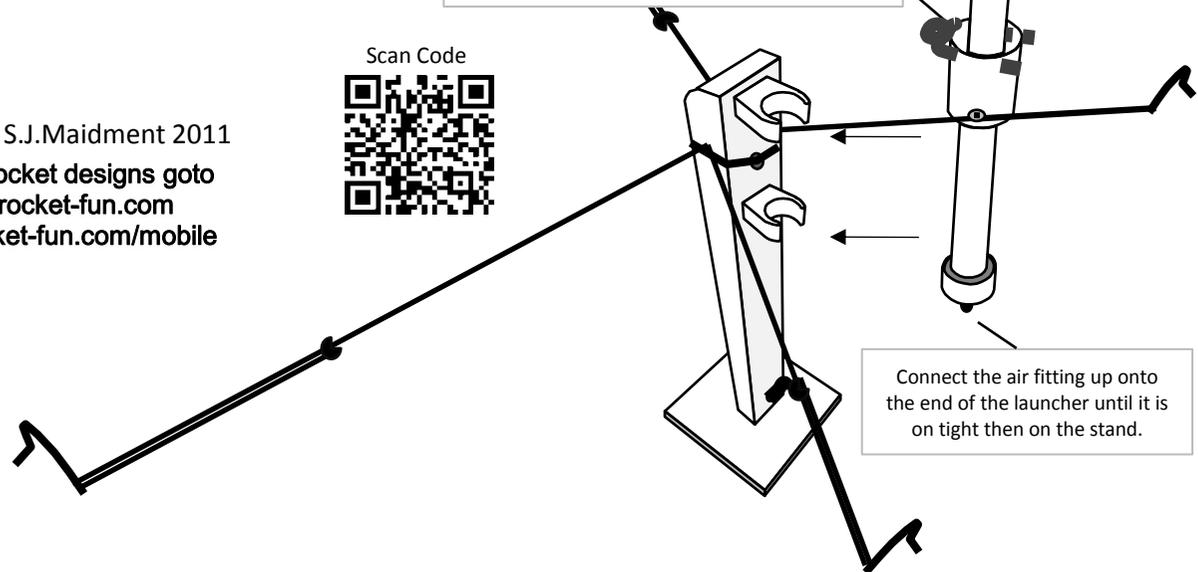
Connect the air fitting up onto the end of the launcher until it is on tight then on the stand.
