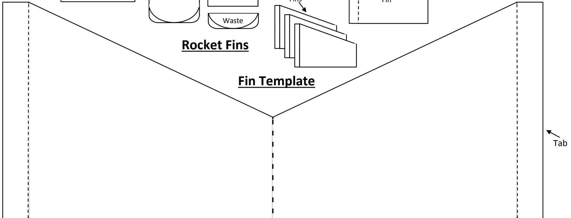
The fins are made out of cardboard from a cereal packet. The fin is in two parts that are stuck or double sided sticky taped together. The two tabs are bent out along the dotted line after scoring with the back of a knife, the tabs are used to tape the fin to the rocket.
