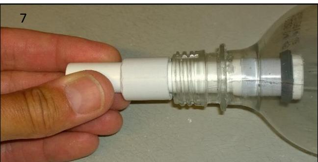
7. Put the 20mm long conduit along the 15mm pex pipe.
