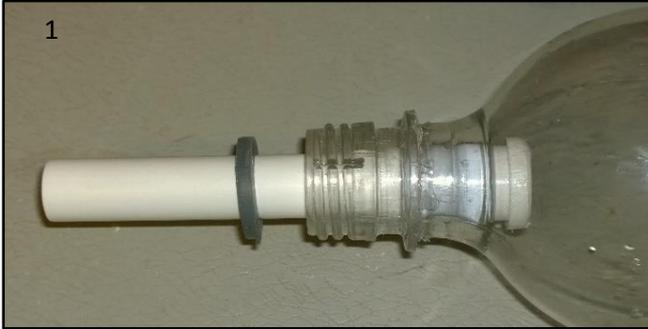
1. Slide the washer down the tube.
