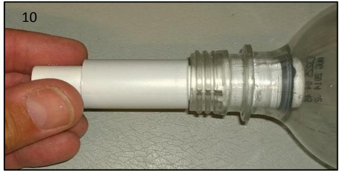
10. Use a spare piece of tube to push the conduit to the washer.
