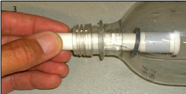
3. Work the washer down the tube.
